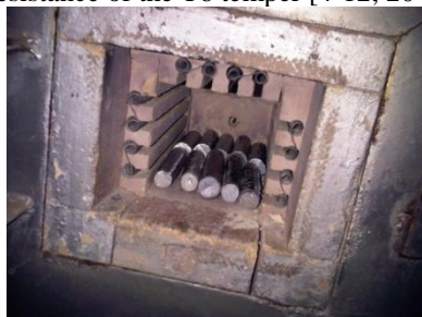
Fig 2. Heat treatment in muffle furnace
